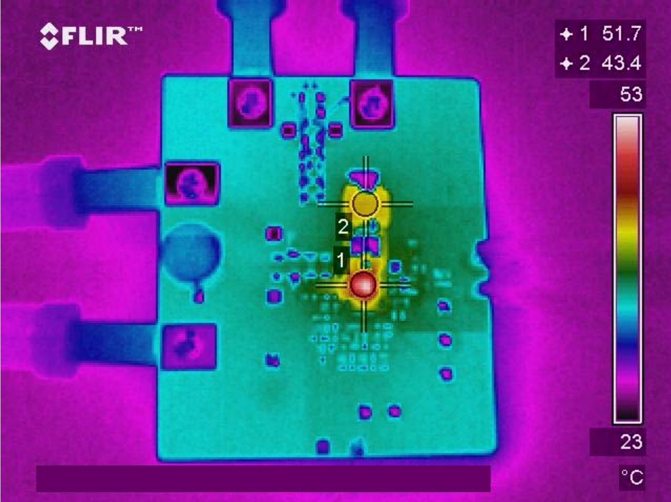
Fig. 18: Thermal Image at 6A load Test points 1 and 2 are IR3856 and inductor, respectively.
