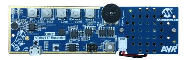
AVR Parrot board implements a voice recorder with ATtiny817. Voice is captured by ADC of ATtiny817 via a microphone, and played back using DAC of ATtiny817. A dataflash device is used to store the acquired voice data.
