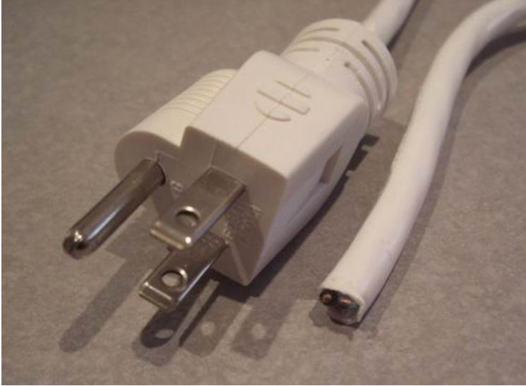
A male US power plug next to the cut off end of the extension cord
